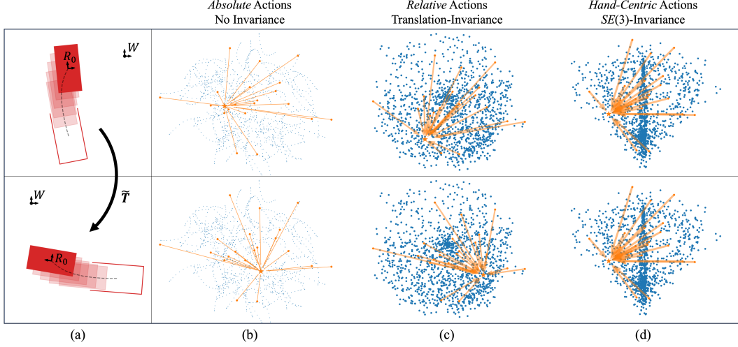
Figure 3: (a) An originally demonstrated action chunk (top) and the same action chunk after applying a rigid transformation (bottom). (b-d) Denoising flows for the 2D position of the first action a_1 of the action chunk (orange), and all training samples for a_1 in the corresponding control representation (blue). (b): Absolute actions – Denoising flow is not invariant; (c): Relative actions – Denoising flow is translation-invariant only; (d): Hand-centric actions – Denoising flow is SE(3) -invariant.
