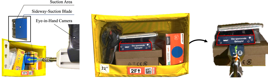
Figure 4: Experimental setup for the real-world visuomotor manipulation task. With an eye-in-hand camera providing RGB-D observations, the task is to insert the manipulation blade into tight gaps and to use sideway-suction to pick thin items from clutter.
